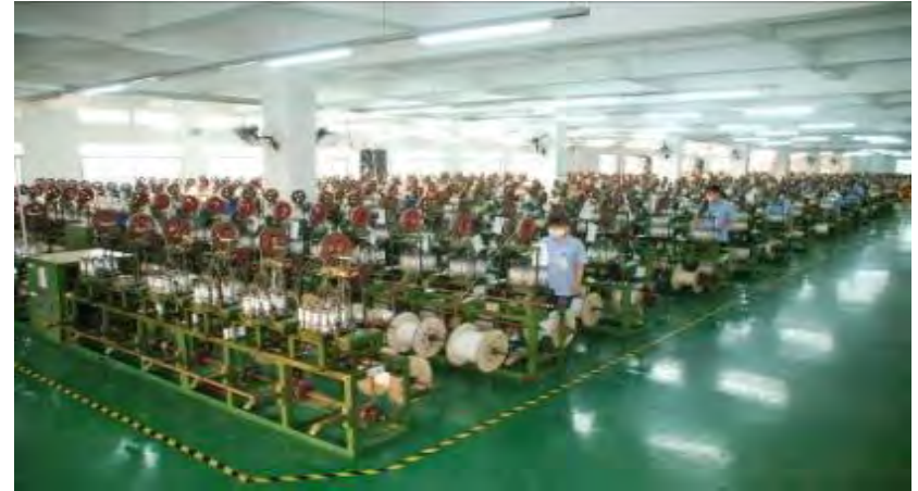
Fiberglass Yarn Braiding
