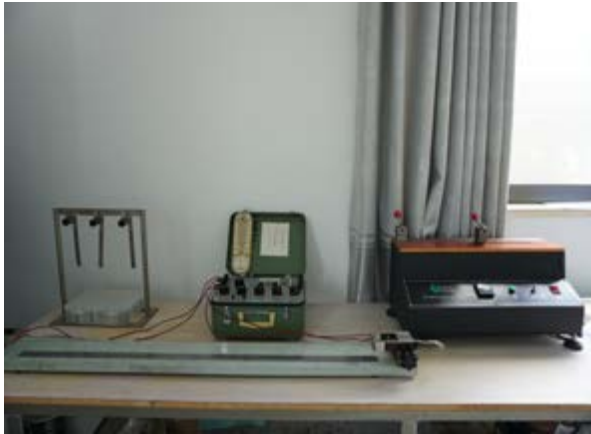
DC Resistance Bridge
