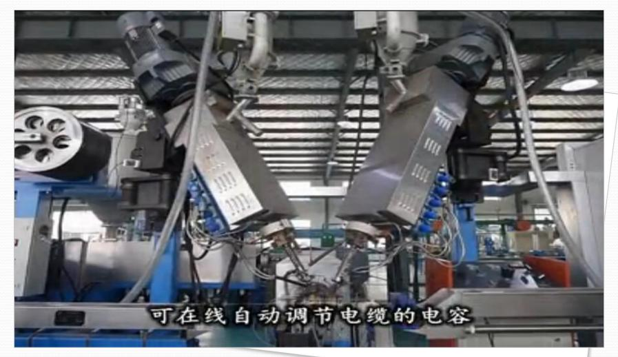
We equipped Italian Sikoraag on line testing system, which can adjust monitor and adjust the electric capacitance, out diameter, eccentricity of the cable. We also equipped Swiss Zumbach testing system series production line, which ensure the high quality of the coaxial cable.
